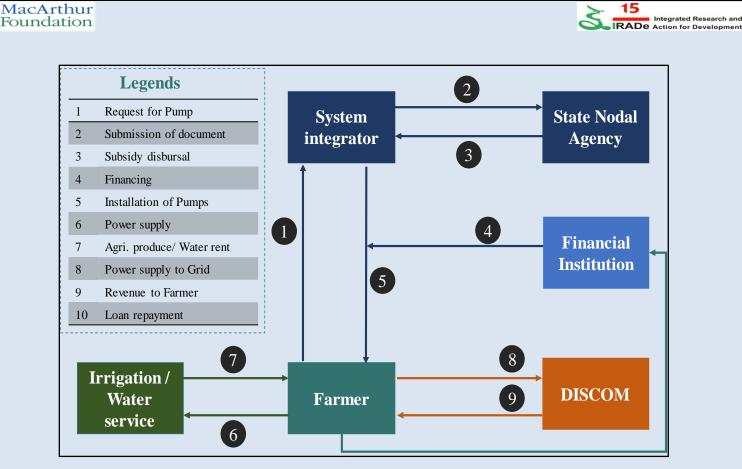
Figure 10: Schematic framework of grid-connected SWP Source: Created by IRADe
